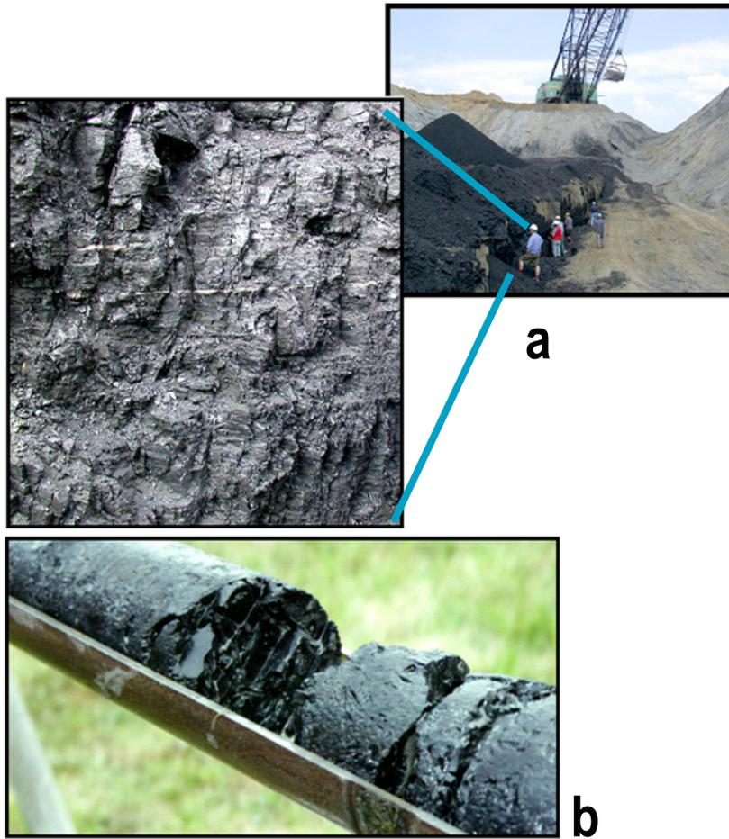
Figure 30. Coal cleat from the Ardley Coal Zone: a) Whitewood Mine, and b) exploration core
