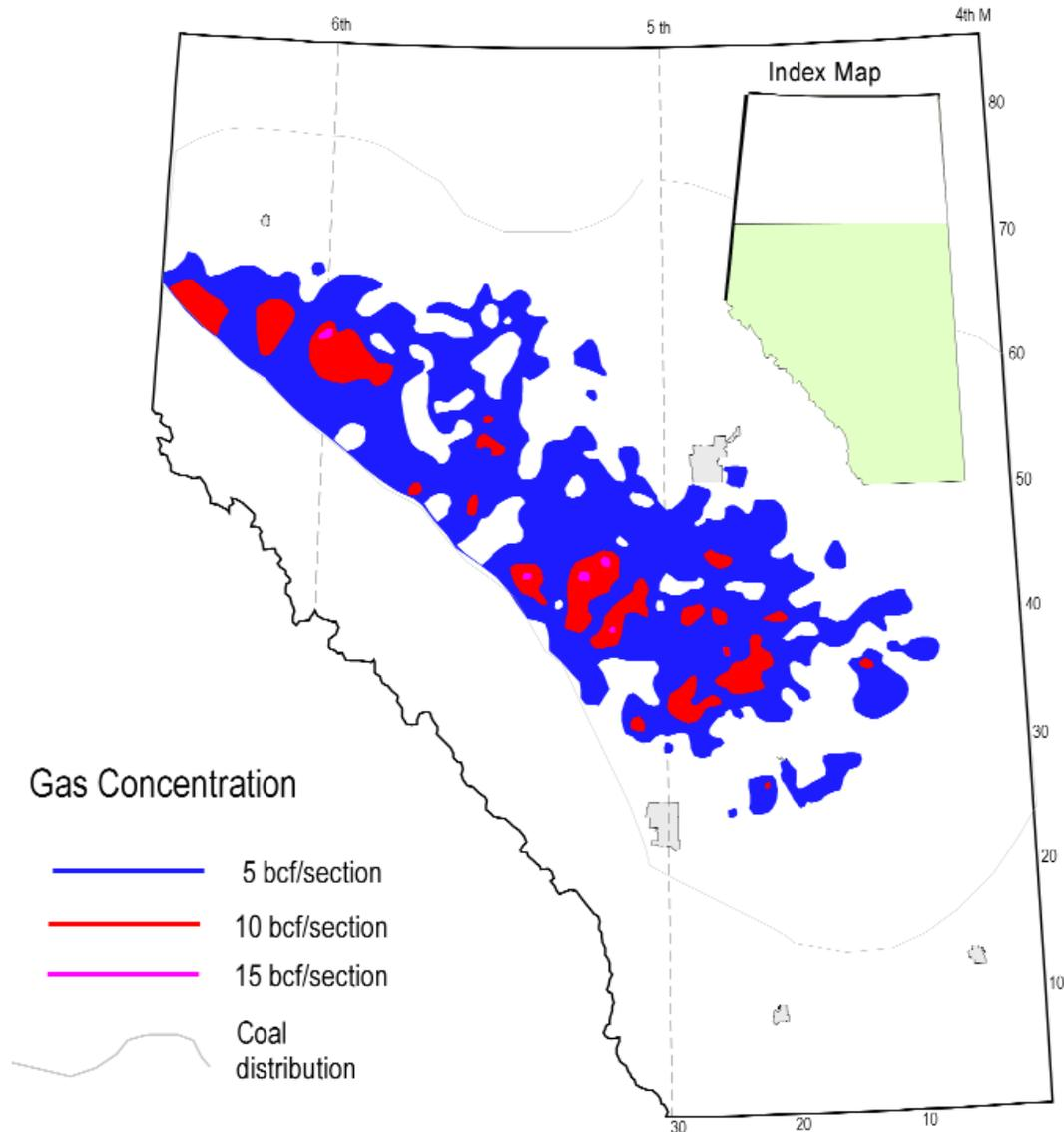
Figure 27. Calculated gas-in-place (in bcf/section), Mannville Coal Zone.
