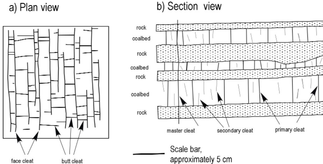
Figure 7. Cleats in coal (modified from Laubach et al., 1998).
