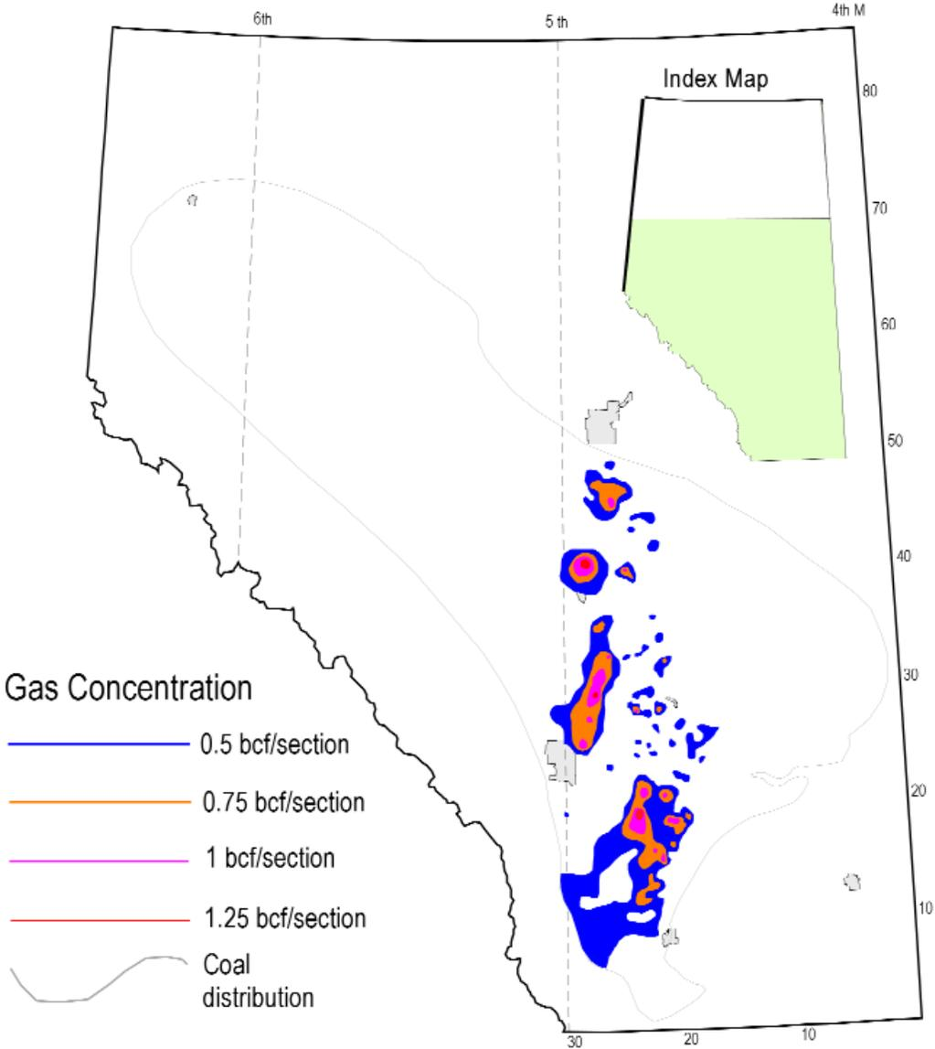
Figure 24. Calculated gas-in-place (in bcf/section), Lethbridge Coal Zone, Belly River Group.
