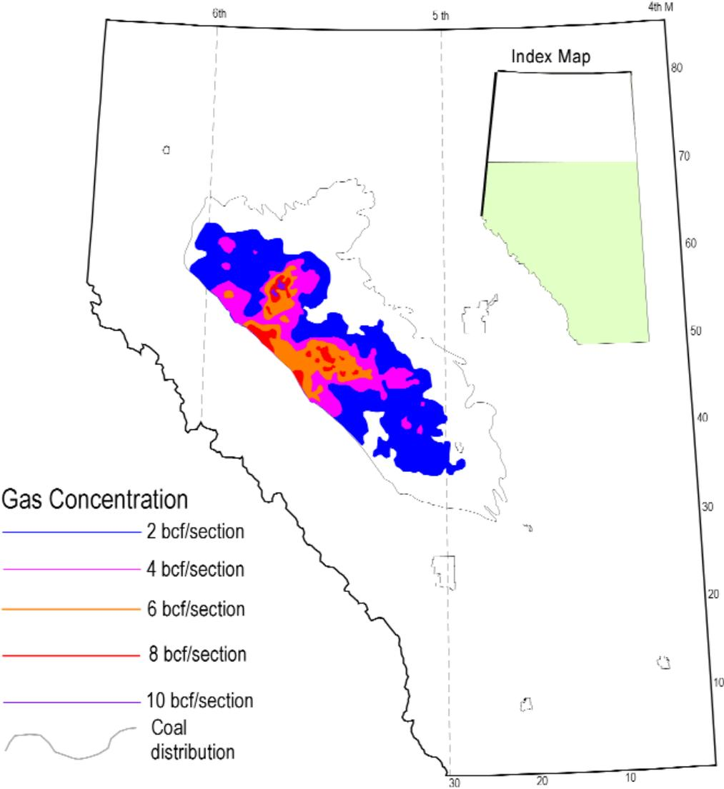
Figure 21. Calculated gas-in-place (in bcf/section), Ardley Coal Zone, Scollard Formation.
