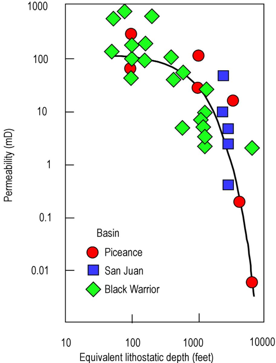
Figure 8. Permeability versus depth (modified from McKee et al., 1988).
