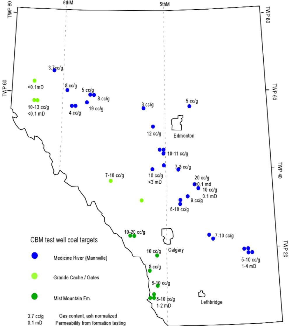
Figure 40. Distribution of CBM wells, gas concentrations and permeability, Mannville and equivalent coal zones.
