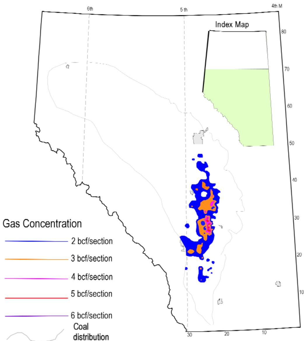
Figure 23. Calculated gas-in-place (in bcf/section), Drumheller Coal Zone, Horseshoe Canyon Formation.
