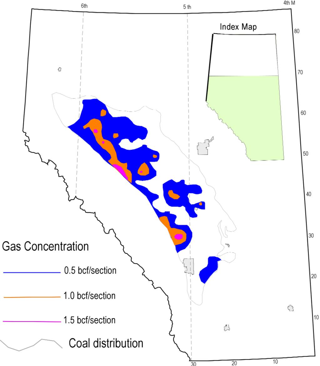
Figure 22. Calculated gas-in-place (in bcf/section), Carbon-Thompson Coal Zone, Horseshoe Canyon Formation.
