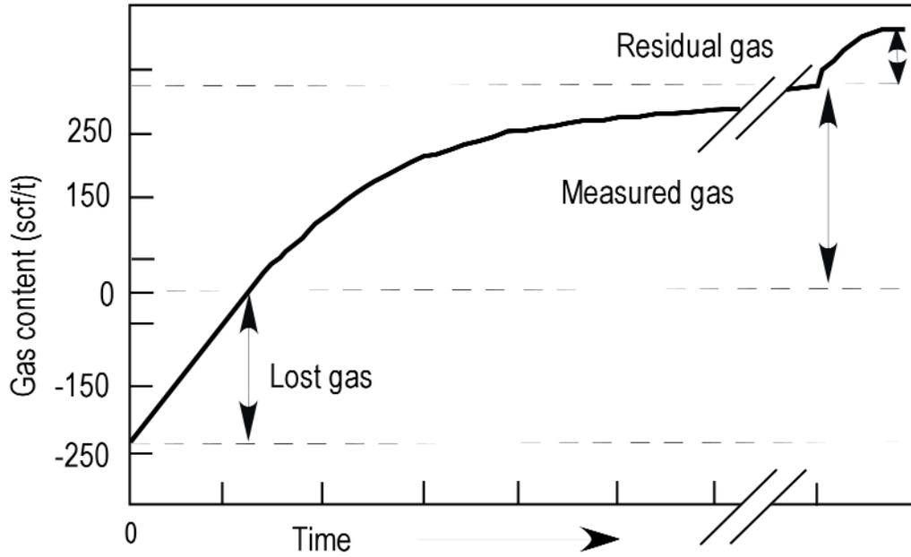
Figure 5. Example of a desorption isotherm plot (modified from McLennan et al., 1995).
