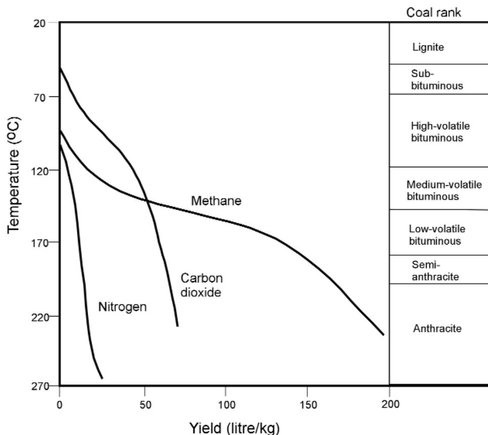
Figure 2. Gas generation potential as a function of coal rank (*modified from Hunt, 1991*).
