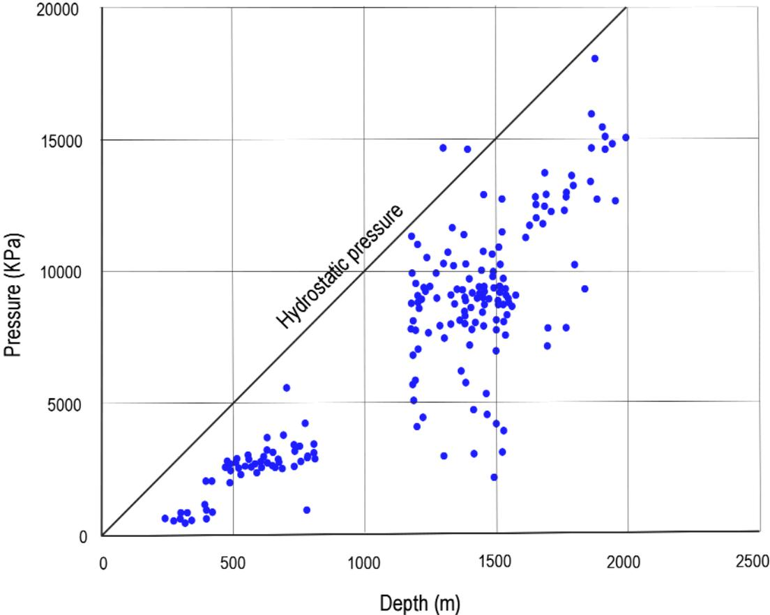
Figure 34. Pressure versus depth, with comparison to hydrostatic gradient, Alberta Plains from oil and gas wells.
