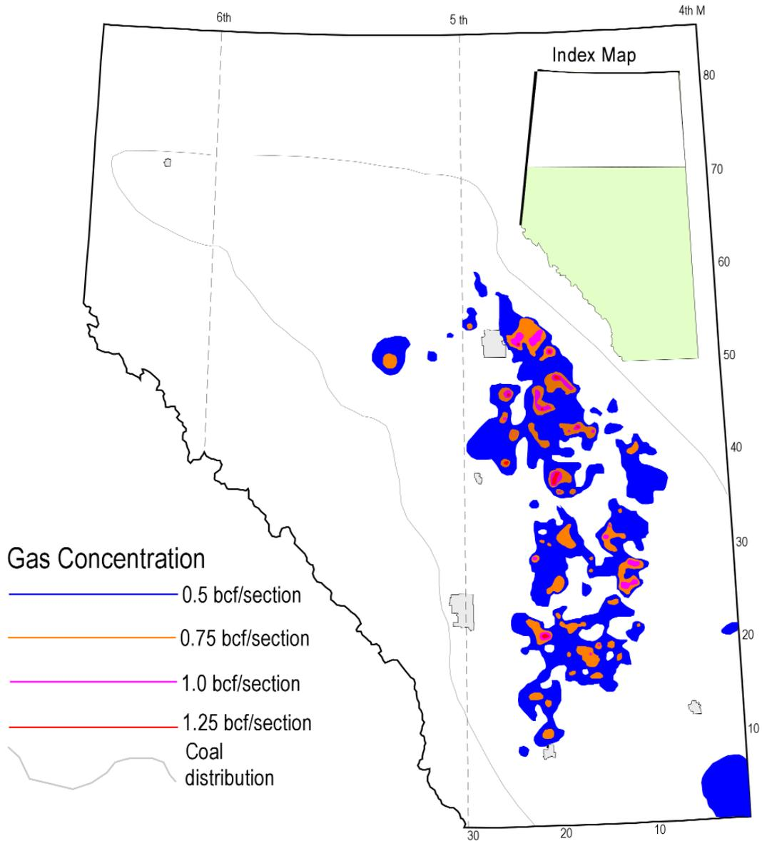
Figure 26. Calculated gas-in-place (in bcf/section), McKay Coal Zone, Belly River Group.
