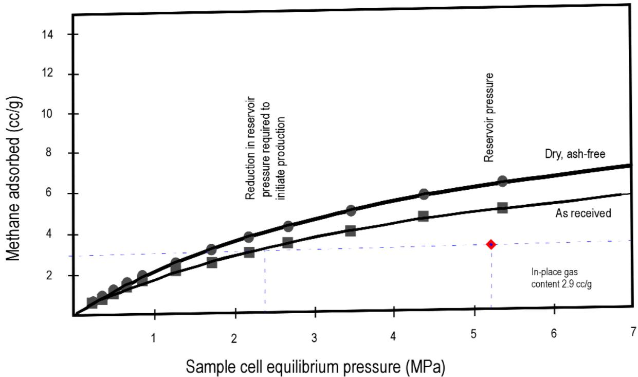
Figure 6. Example of an adsorption isotherm plot.
