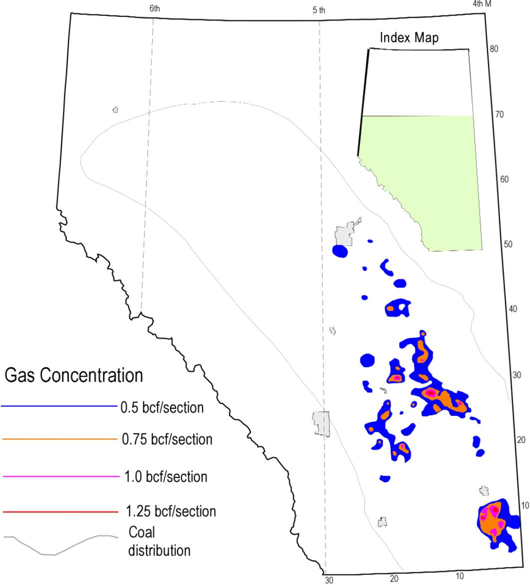
Figure 25. Calculated gas-in-place (in bcf/section), Taber Coal Zone, Belly River Group.
