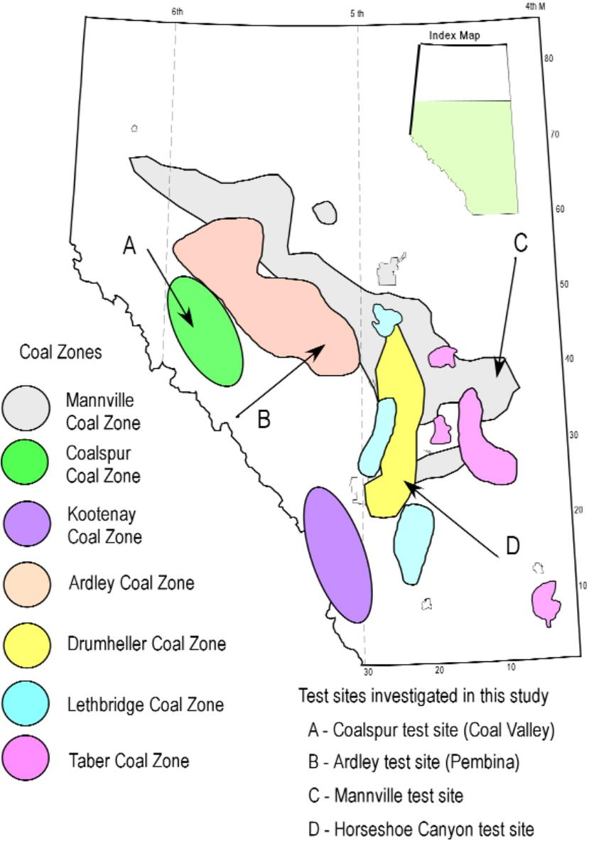
Figure 28. Areas with potentially favourable coalbed methane exploration potential, Alberta Plains, and test site locations investigated in the current study.
