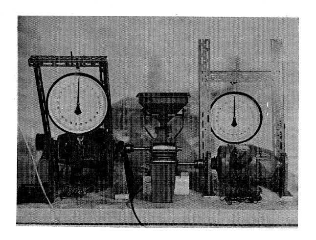
Figure 1 The Research Council of Alberta grindability apparatus.
