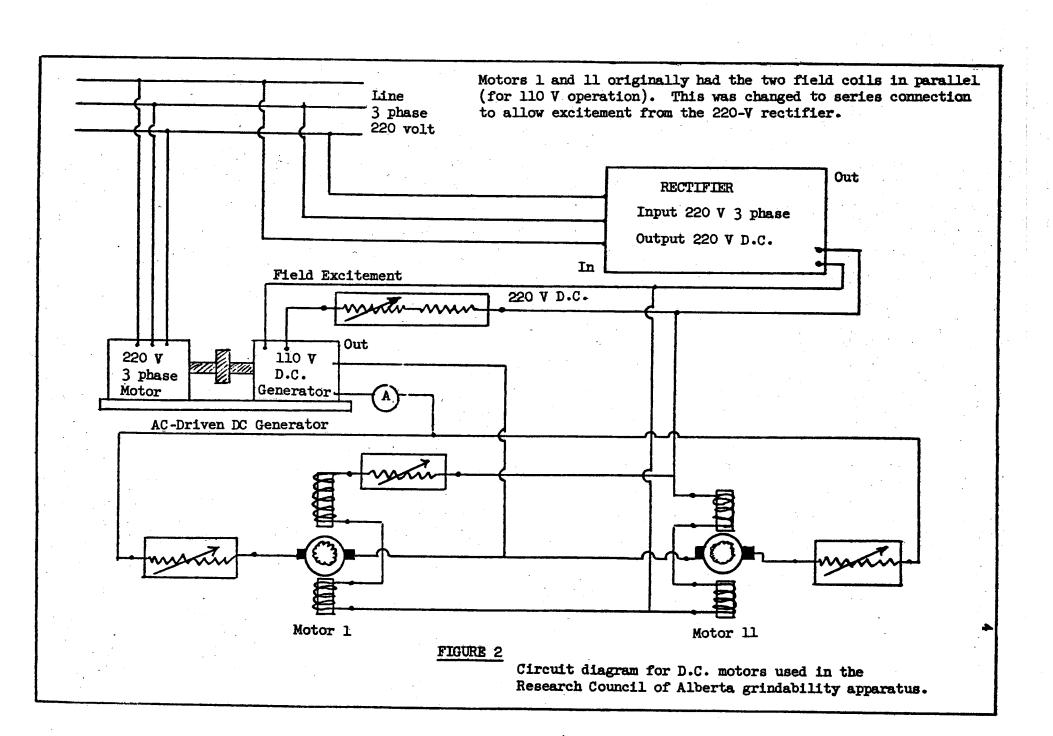
rolls by springs. Each roll is turned by a motor attached to a shaft by means of a rigid coupling. Each motor is suspended in ball bearings so that the torque developed in the motor can be measured on a dynamometer attached to the motor by an arm 1 foot in length; D. C. shunt motors are used, and the electrical arrangement is shown in Figure 2.
