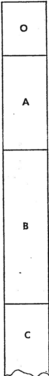
Figure 1. A sketch of a soil profile showing major soil horizons and a brief outline of difference in properties.
