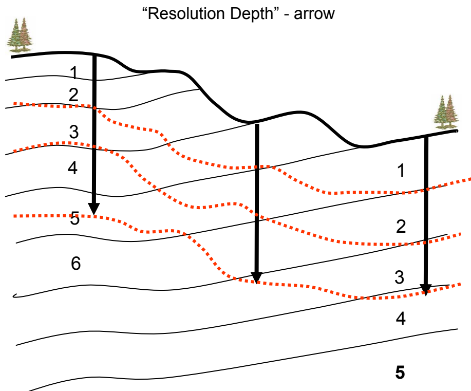
Figure 5: The cartoon of Figure 4 repeated here to show how the inversion layers (dotted red lines) might cross the model. However, one would expect the distinct resistivities of the actual layers to be mapped in each of the inversion layers where they cross the actual layers.
