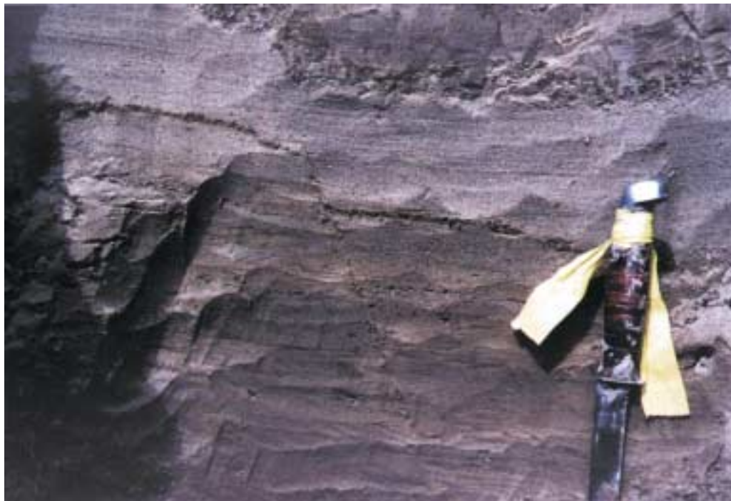
PLATE 5.8 - Micro-faulting due to loss of support..
