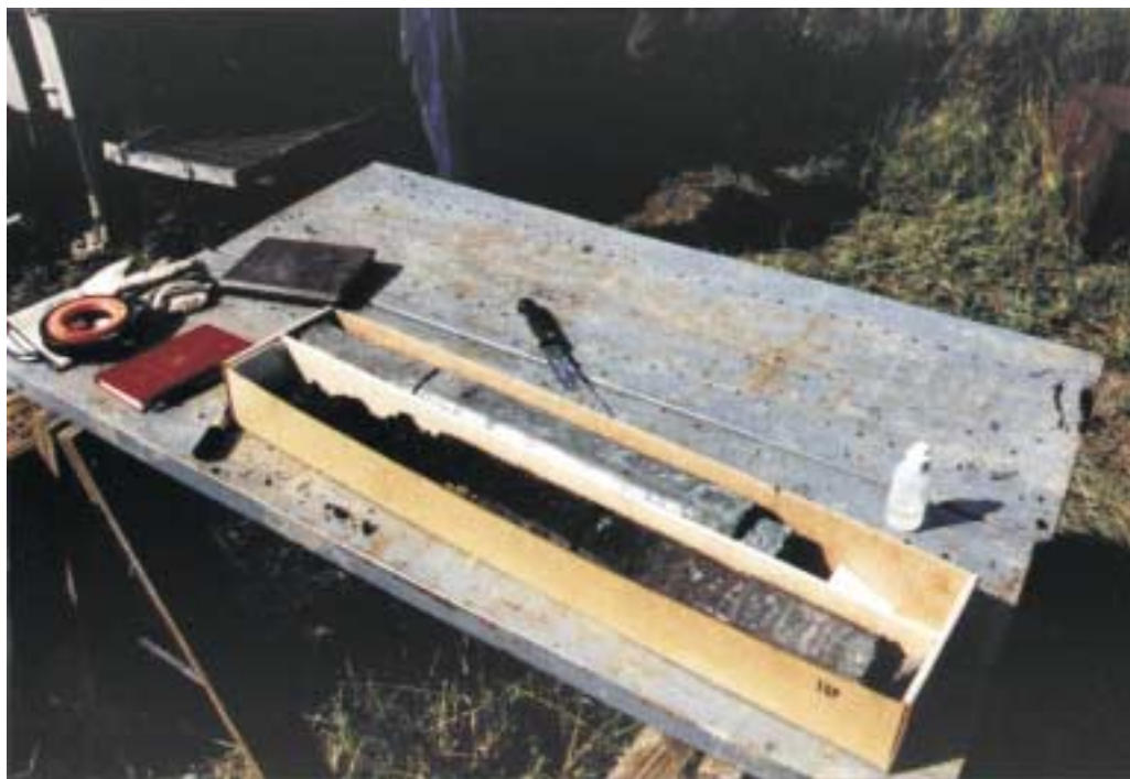
PLATE 3.2 - Core description set-up.
