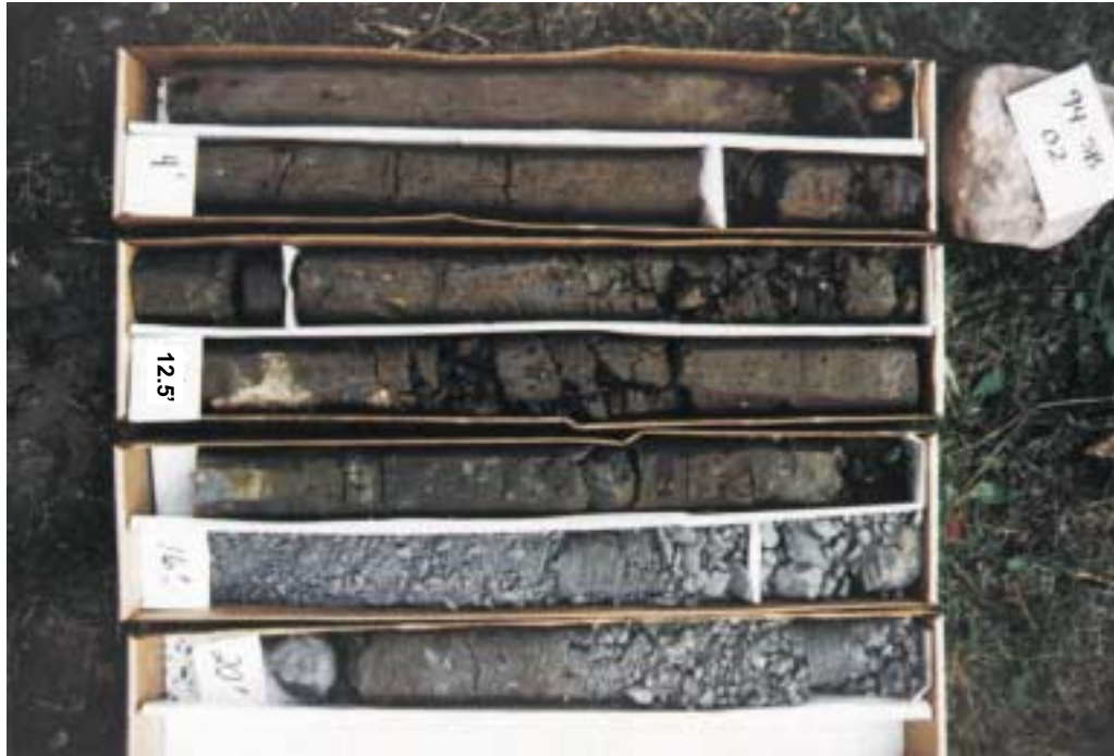
PLATE 6.7 - Oxidized supraglacial and meltout tills (sub-units C2 and C3) in borehole 94-SAB-02.
