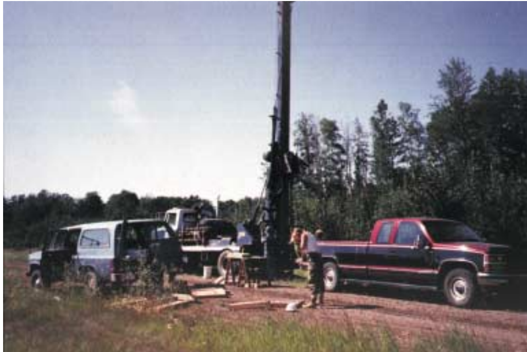
PLATE 3.1 - Auger drill rig set-up.
