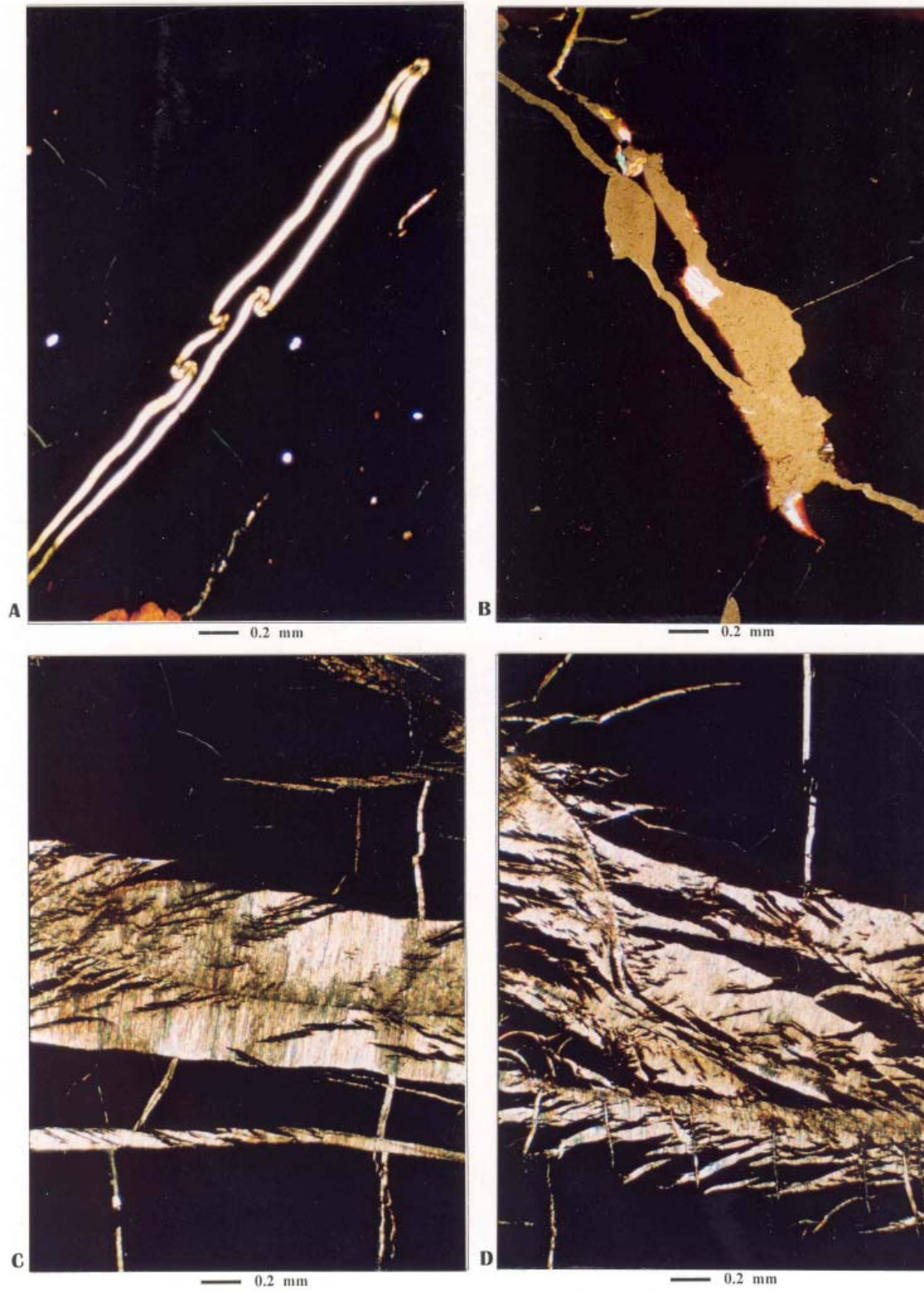
Figure 1. Photomicrographs of thin sections of coal. A) Enigmatic liptinite (?) maceral included in vitrinite. B) Cavities with small calcite crystals. C) Cluster of calcite veins and cleats. D) Cluster of calcite veins and cleats.
