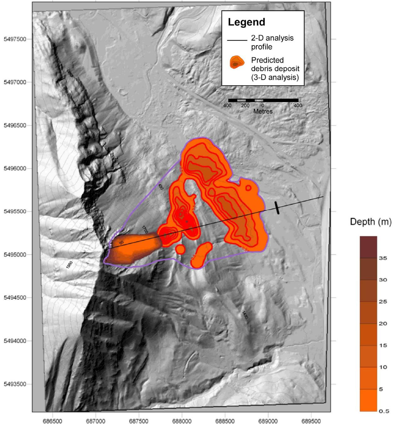
Figure 15. DAN3D three-dimensional forward prediction of the 6.6 million m<sup>3</sup> slide from the lower portion of South Peak (from Hungr Geotechnical Research, 2008).
