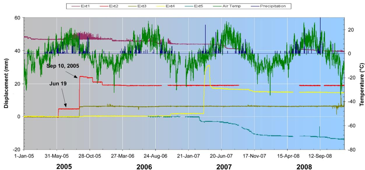
Figure 7. Plot of displacement versus time for extensometers, South Peak, Turtle Mountain.
