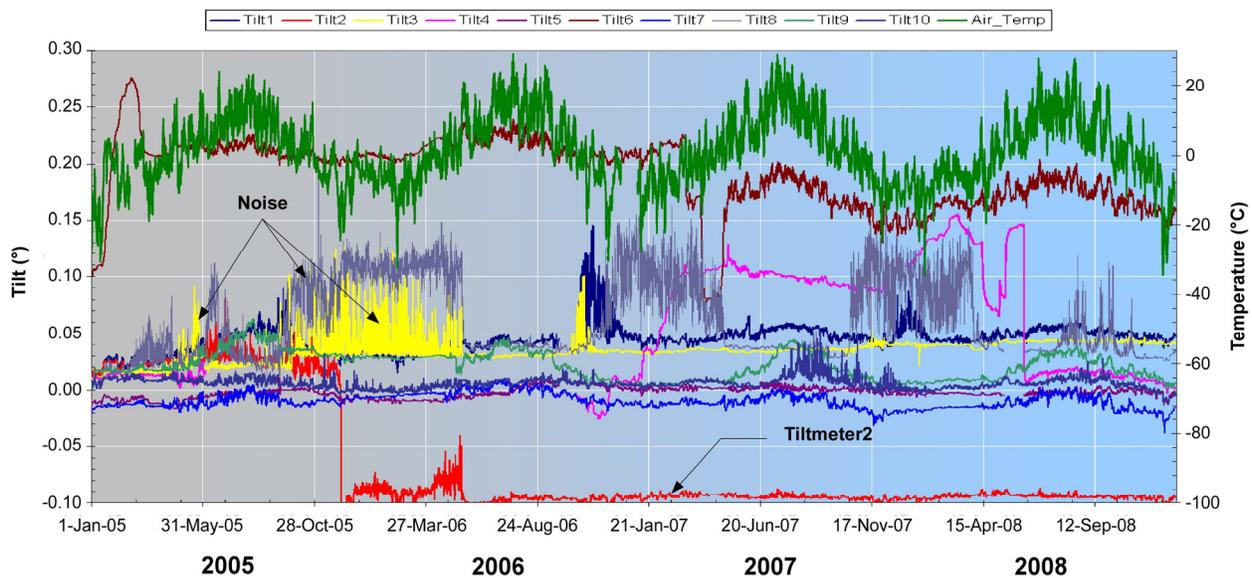
Figure 6. Plot of tilt versus time for tiltmeters, South Peak, Turtle Mountain.
