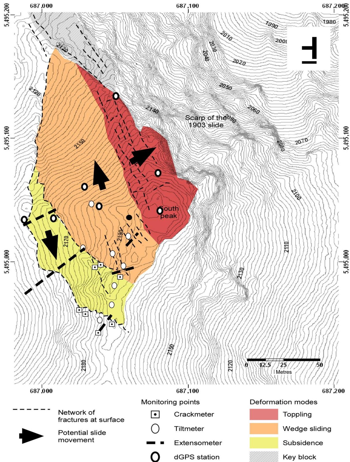
Figure 12. Location of monitoring points relative to the four main zones of deformation observed on the South Peak of Turtle Mountain.
