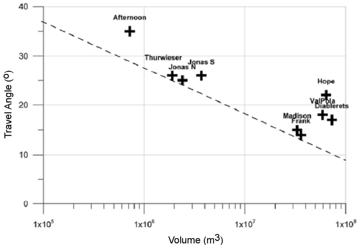
Figure 14. Calibration analysis: correlation between landslide volume and the back-calculated bulk friction angle (from Hungr, 2008).
