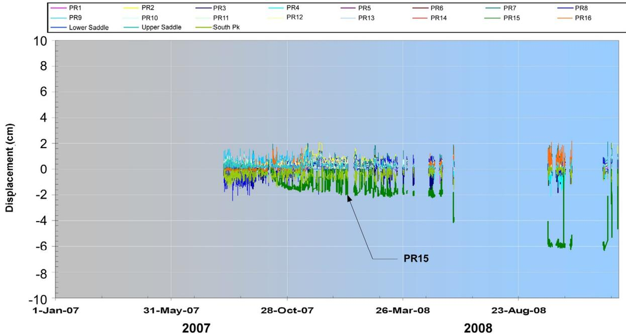
Figure 9. Plot of displacement versus time for prisms at Turtle Mountain.
