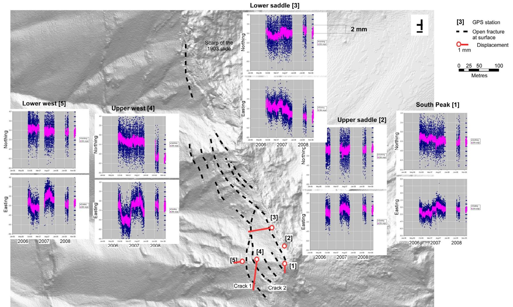
Figure 8. Surface displacements derived from dGPS stations during the period 2006–2008: horizontal component of the surface-displacement vectors plotted on a map of the South Peak of Turtle Mountain (red lines). The displacement vectors of the dGPS stations are absolute, since they reference an external co-ordinate system. dGPS stations: [1], South Peak; [2], Upper saddle; [3], Lower saddle; [4], Upper west; [5], Lower west.
