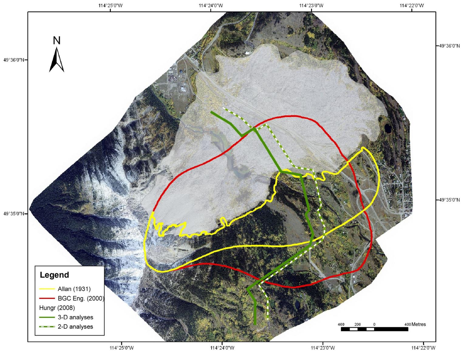
Figure 17. Summary of maximum run-out extent results from piecemeal failure analysis by Hungr Geotechnical Research in 2008, in relation to previous single-mass failure estimates (Allan, 1931; BGC Engineering, 2000).
