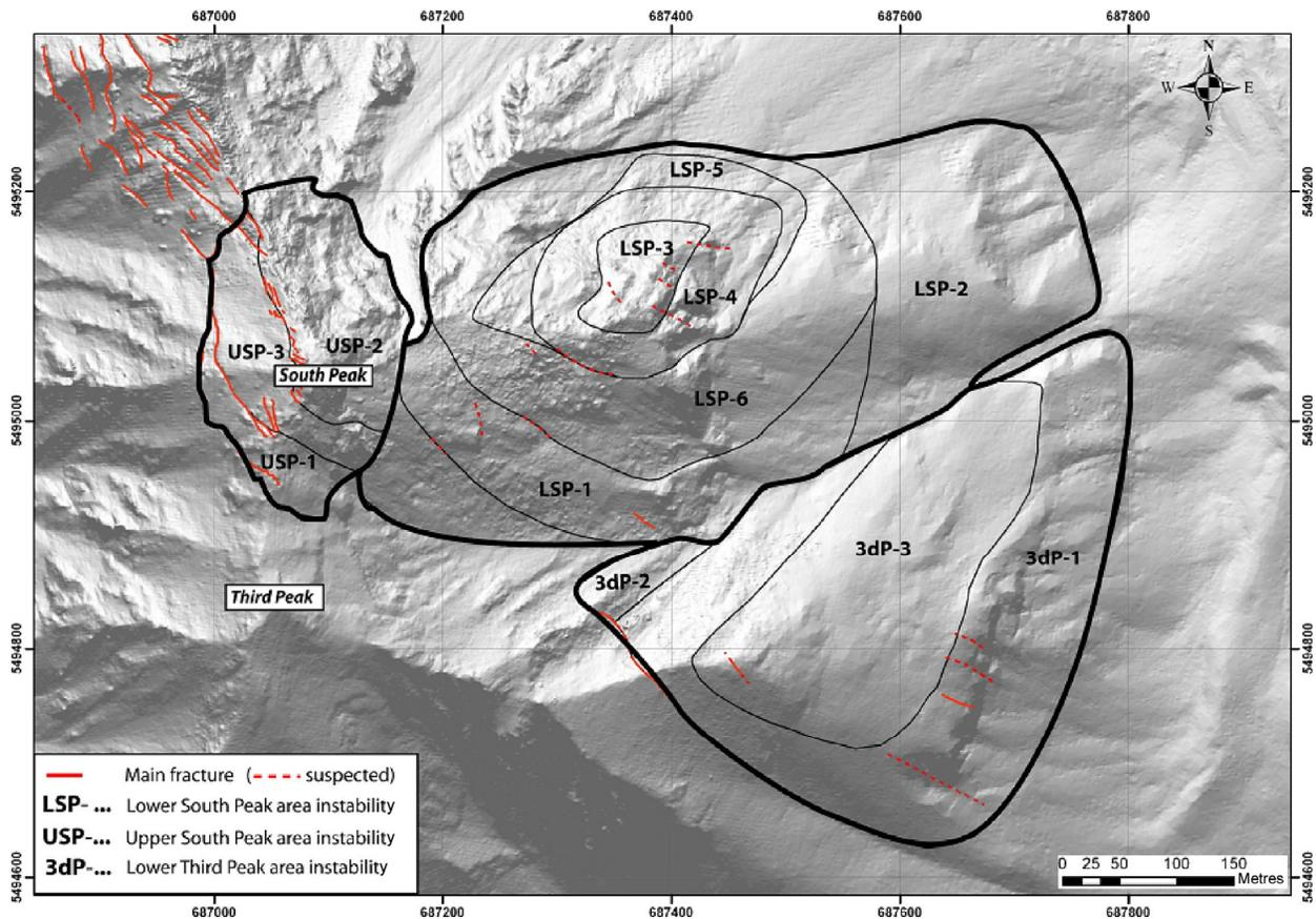
Figure 13. Instability zones in the South Peak and Third Peak areas identified by the detailed structural mapping and kinematic analysis (from Pedrazzini and Jaboyedoff, 2008)
