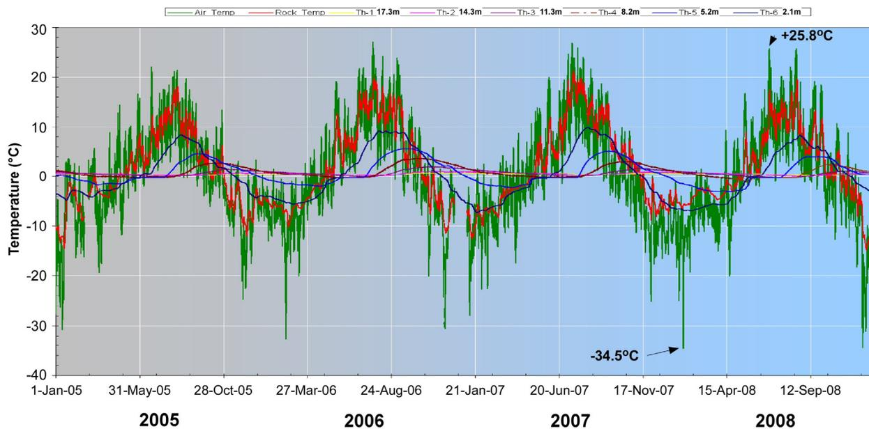
Figure 10. Air temperature and variation of rock temperature with depth in the borehole at the top of South Peak, Turtle Mountain, 2005–2008.
