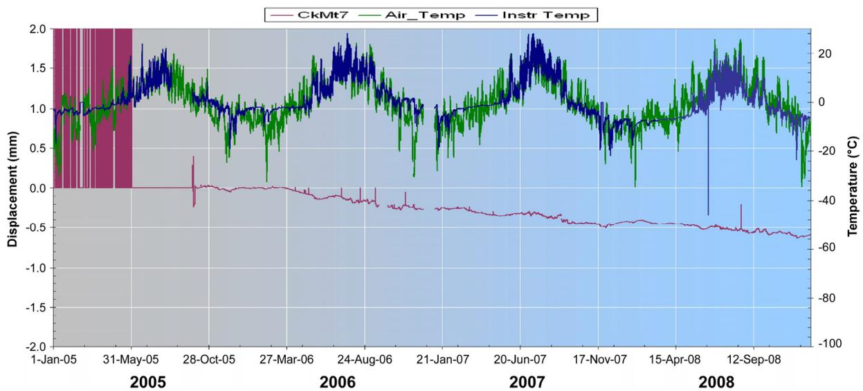
Figure 5. Plot of displacement versus time for crackmeter CM-7 of set C, South Peak, Turtle Mountain.
