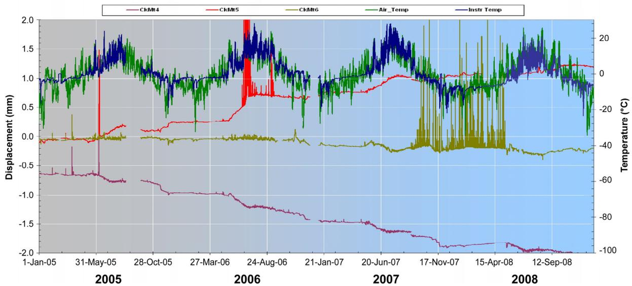
Figure 4. Plot of displacement versus time for crackmeter set B, South Peak, Turtle Mountain.
