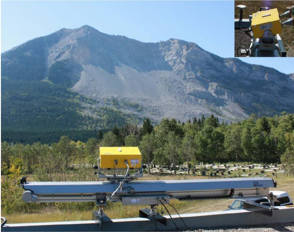
**Figure 13.** The IBIS-L GB-InSAR system is installed on a rooftop, facing the unstable slopes on Turtle Mountain. The farthest point on the mountain crest is approximately 3200 m away.
