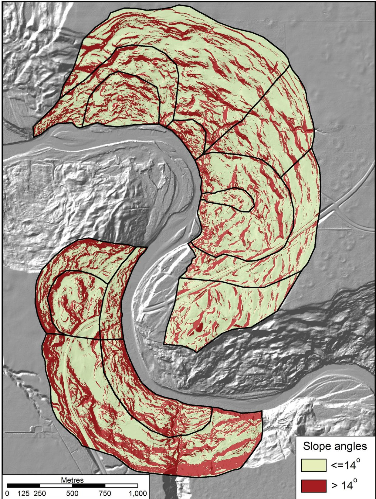
Figure 6. Slope angle derivative map showing the distribution of slope angles for each landslide.
