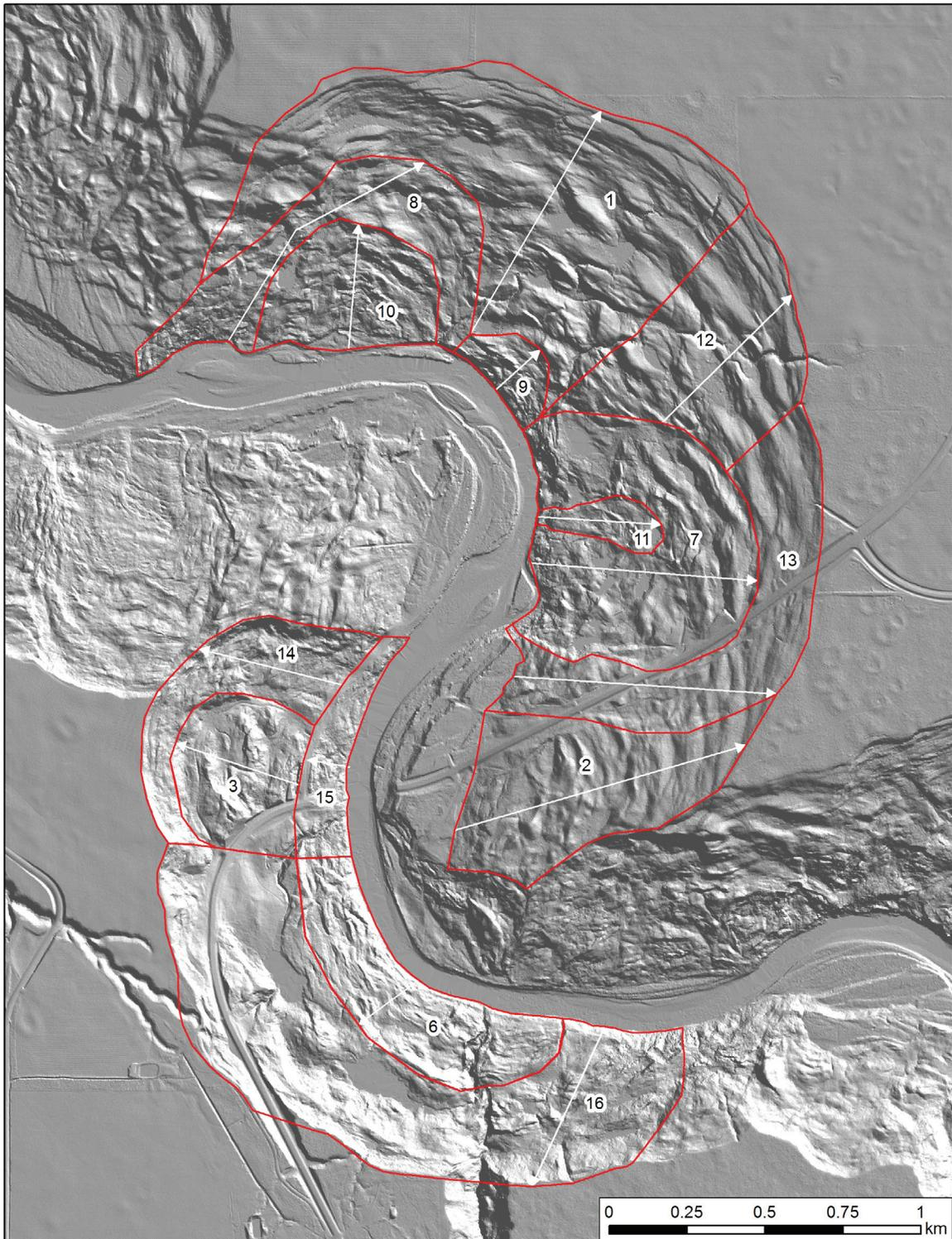
Figure 11. Key map showing landslide boundaries, identification numbers, and profile lines.
