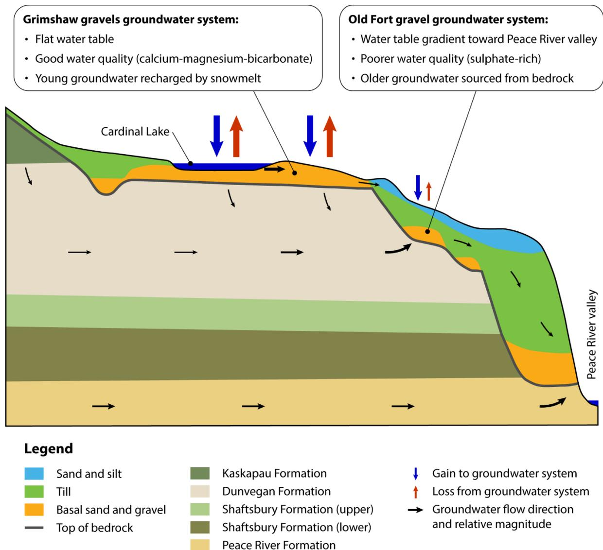
**Figure 13. Conceptual model of the Grimshaw gravels aquifer system, illustrating terraced groundwater systems, major gains (e.g., recharge) and losses (e.g., evapotranspiration, pumping) for the groundwater budget. Shaftsbury gravel not included due to insufficient data.**
